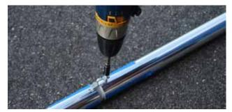
**STEP 7** - Attach the bungee cord loop with one self tapping screw on each piece (on either side of the seem). See predrilled holes.
