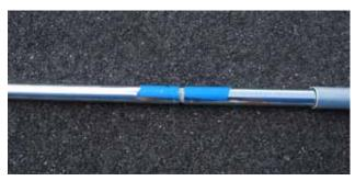
**STEP 5** - Remove the vice grips from the sleeve and then stand the upright on end and tap the end on a solid surface until the two pieces are joined together
